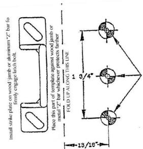
Cut out template along this line CAUTION: locate installation so that latch will not hit entrance lock. Drilling template Follow these instructions for correct location of installation holes.
