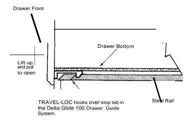
The **Delta Travel-Loc** can be incorporated with the **Delta Glide 100 Drawer Slide System.** The **Travel-Loc** eliminates the need for special cabinet construction or expensive latches.
